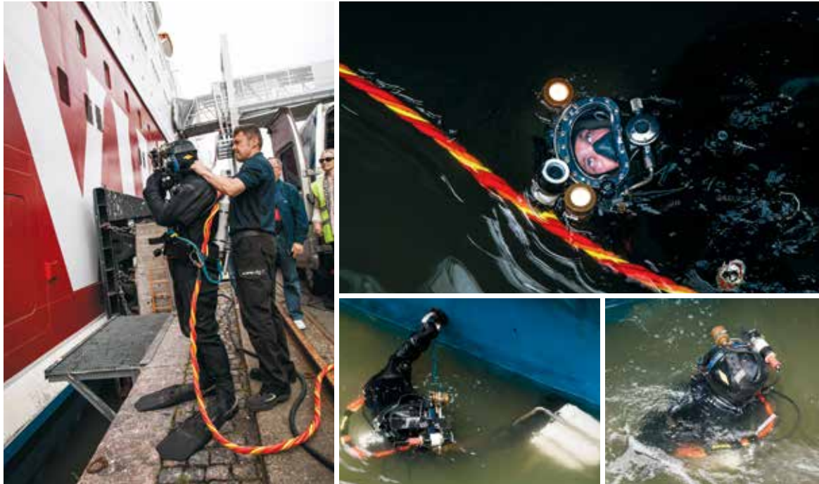
The hulls of the vessels are brushed by divers several times each year. All growths loosened from the hulls during brushing are collected into a separate container, which is then brought ashore for further treatment.
