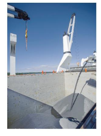
> Pellets - the iron ore is crushed and ground to a powder and the iron ore is separated. Afterwards the iron ore is rolled together to form 8-15 mm round balls with different additives to improve the product's properties. These balls are sintered at 1,100-1,200 degrees to form a solid product. The product is then used directly in the blast furnaces.
