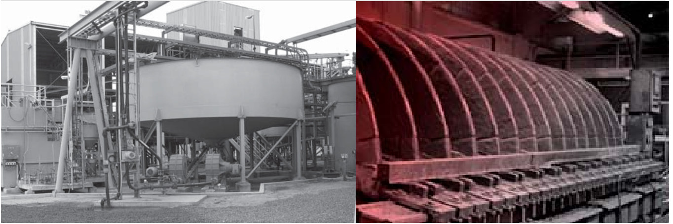
The Angas Mine one the Terramin Australia Pty Ltd's base metal projects is equipped with Larox Ceramec CC30 filters, which are used for zink dewareing.
