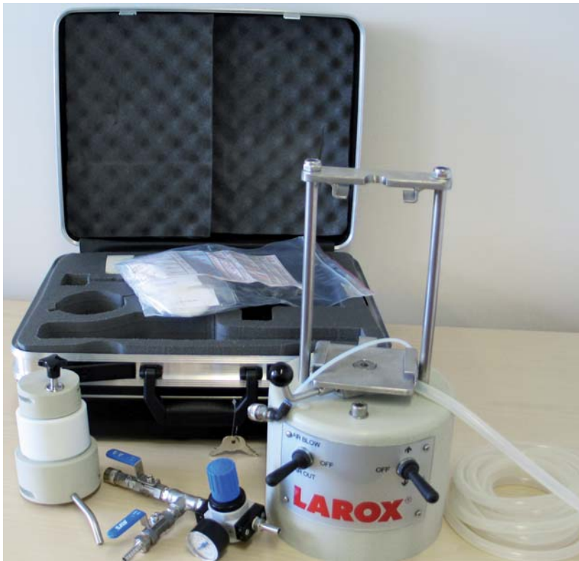
The complete Labox 25 test unit.
