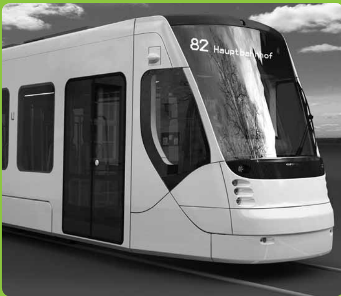
A newly developed tram made of stainless steel for street traffic.
