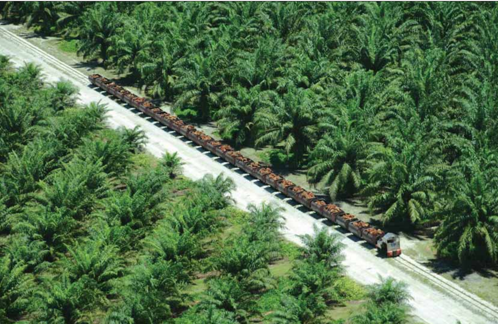
UPB's unique light railway system showing a diesel locomotive pulling a train of fruit cages containing freshly harvested fruit bunches. UPB's railway system stretches over 500km and is one of the main contributing factors for its superior quality crude palm oil.
