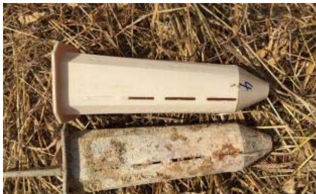
Initial trials for a new, biobased and biodegradable root protection cone for rubber trees by Corbion, Maxrich and Global Bio-Polymers have been promising
