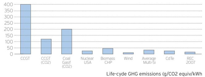
**Figure 1. Life-cycle greenhouse gas emissions per kWh for different technologies currently being considered in the work to lower emissions of greenhouse gases. CCGT = Combined Cycle Gas Turbine, (CO2) implies a power plant with carbon sequestration and storage, CHP=Combined Heat and Power, CdTe=PV power made from Cadmium Telluride modules. Most data is from 2005 production.**
