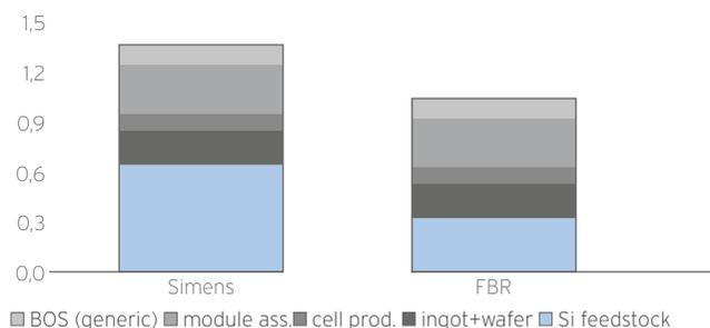
Figure 3: Energy Pay-Back Time for a PV system made by REC with modules using Siemens- or FBR-type feedstock. The different colors represent the contributions from the silicon, wafer, cell, module and BOS share of the total system.
