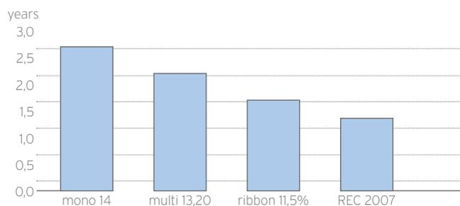
Figure 2. Energy Pay-Back time (in years) of solar systems for the three main silicon-based PV technologies in 2005 compared to REC 2007. The solar systems are assumed installed in Southern Europe, with about 1700 sun hours per year.
