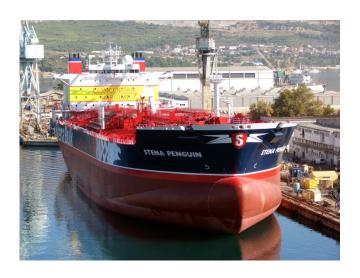
The first P-MAX tanker was delivered in 2005 from Brodosplit Shipyard. The tankers have double hulls, optimum corrosion control, two engine rooms with full water and fire integrity and two separate propulsion systems. Superior manoeuvrability and an integrated bridge layout facilitate safe navigation in narrow channels. The *Stena Penguin* is the second tanker in the series with ice class 1A.
