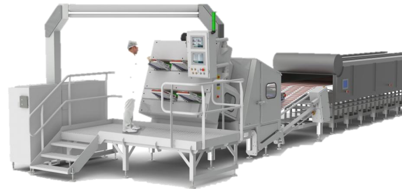
IBS 4600 – the world's first 4-blade, 4-lane bacon slicer – has enjoyed great success since its launch last year
