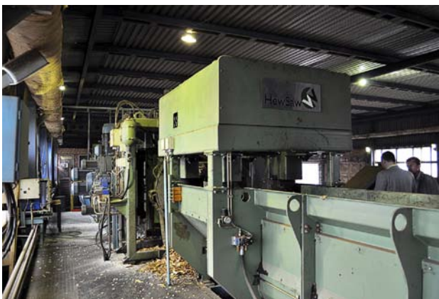
RusForest Ust-Ilimsk: The HewSaw R200 sawline
