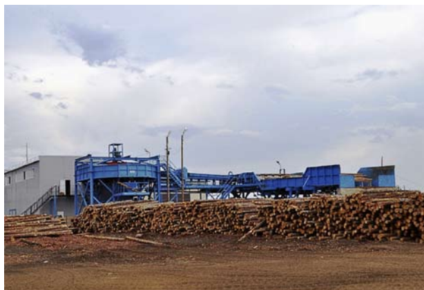
Boguchansky LPK: Overview of the sawlog table and log turner
