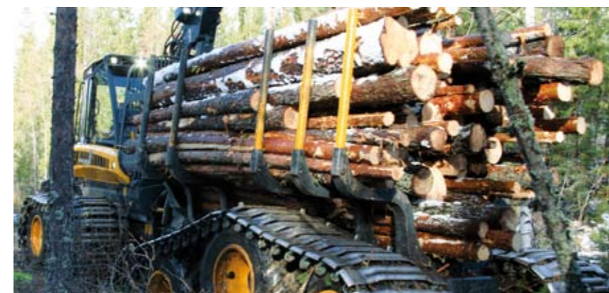
A ten-wheel forwarder solution for harvesting in poorly supporting terrain was launched in October.
