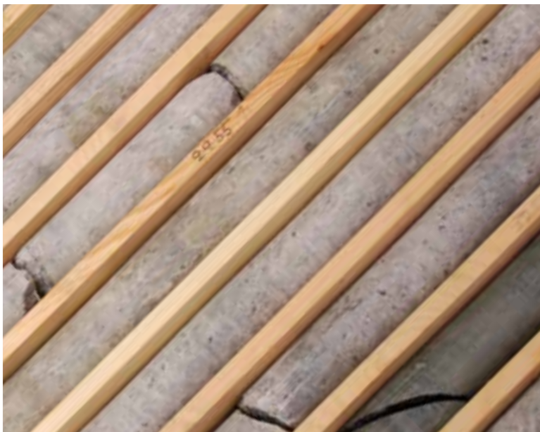
The cores are logged and sampled. The results form the basis of the mineral resource estimation.
