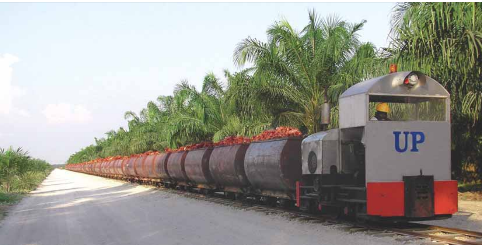
UPB's unique light railway system showing a diesel locomotive pulling a train of fruit cages containing fresh fruit bunches. UPB's railway system stretches over 500 km and is one of the main reasons for its superior quality crude palm oil.
