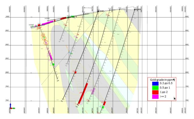
Picture 4. Cross section along drill profile 40. New mineralized intervals following the resampling program are marked with circle.
