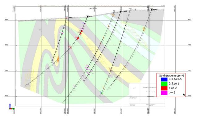
Picture 7. Cross section along drill profile 57
