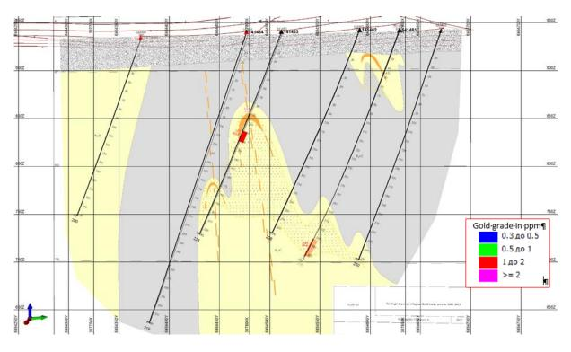
Picture 2. Cross section along drill profile 16
