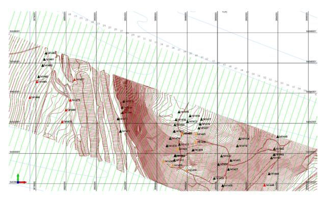
Picture 1. Plan view of Krasny South site – recent drilled holes marked with red color, resampled holes marked with orange color
