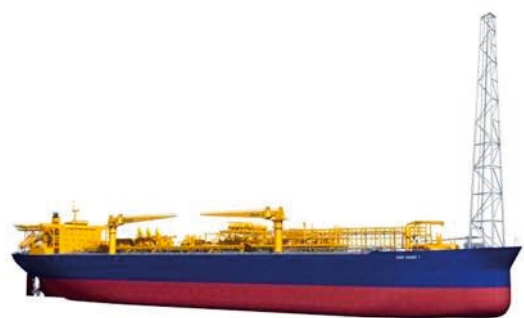
The Aker Smart 1 FPSO (Floating Production, Storage and Offloading)
