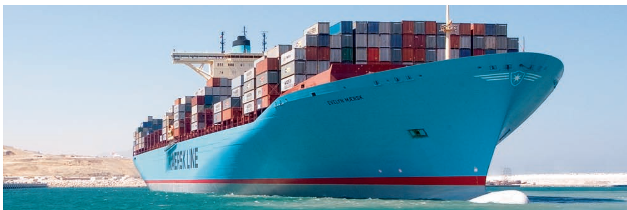
With a capacity of 11,000 TEU EVELYN MAERSK is one of the world's largest container vessels along with the other seven in the series. The PS-Class sets new standards within size, as well as environment and safety.
