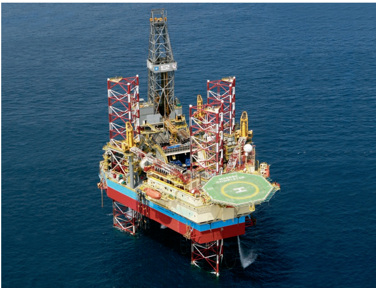
MAERSK COMPLETER is the first of two identical jack-up rigs and the first of Maersk Contractors' new C-Class. The rig can drill on depths of 375 feet (115 metres) and has a drilling depth of down to 30,000 feet (9,144 metres).
