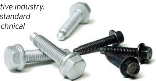
Screws with a guiding pin makes assembly easier as the pin both helps to locate the hole and straighten up the screw. Guiding pins improve assembly efficiency and reduce errors and quality defects.
