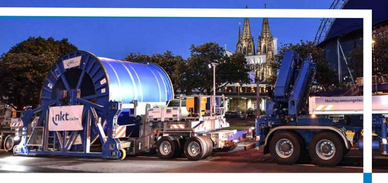
400kV ground cable on a 25 tonne drum being transported through Cologne, Germany. The cable made up part of the connection between a new gas and steam power plant and the German grid over a distance of 9 km - at present the longest 400kV ground cable connection in Germany
