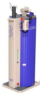
The Alfa Laval Aalborg High Pressure Natural Circulation (HPNC) steam boiler is a high performance boiler developed to comply with the rigorous specifications of the food and vegetable industry, by ensuring high quality and reliability throughout the plant life time. The high pressure boiler is supplied in 9 different standard sizes, with steam effect ranging from 125 to 2,500 kW. The standard
