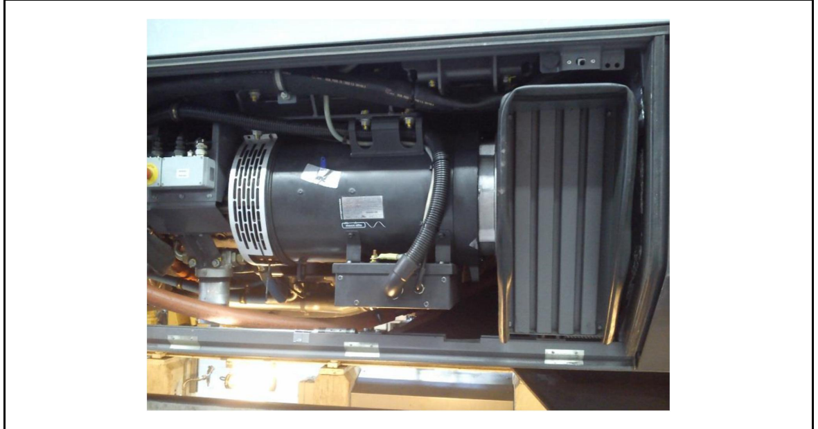
figure 10-18: Alternator with the new air outlet grid (left side) (Shown without side skirt) (A2, 180)
