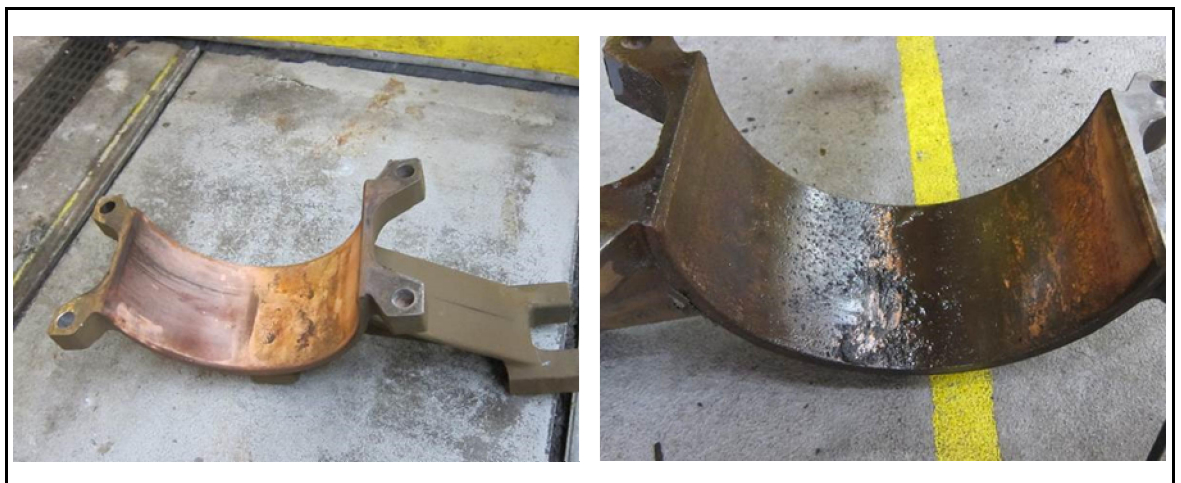
figure 10-9: Pictures of axle box lower parts with fretting corrosion marks
