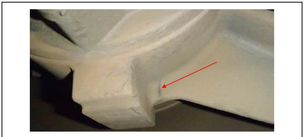
figure 10-8: Cracked primary damper supports under the damper support arm
