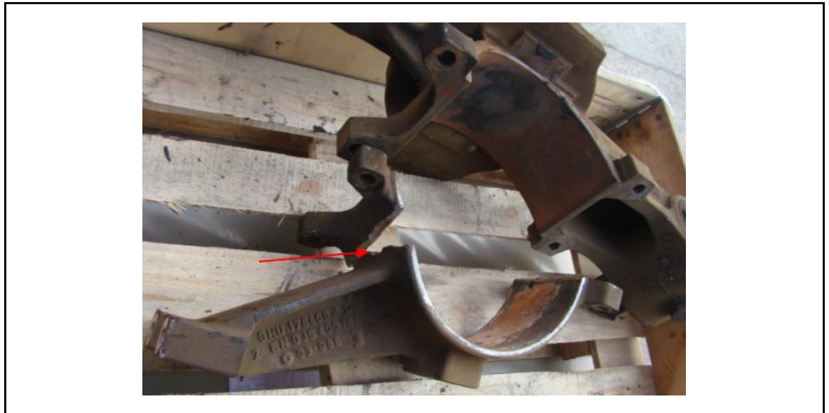
figure 10-7: Fractured primary damper supports above the damper support arm
