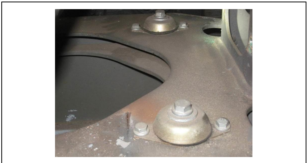
figure 10-19: Damaged rubber element for the fixation of the main hydraulic pump (PROSE)
