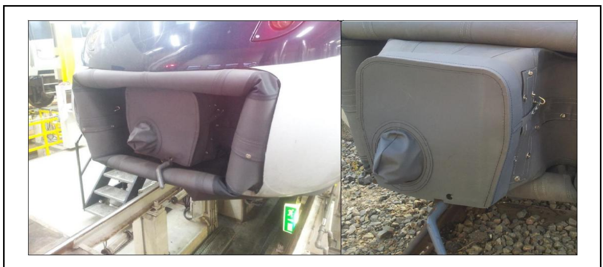
figure 10-1: New gaiter; left picture: coupler retracted; right picture: coupler extracted (A2, 222)
