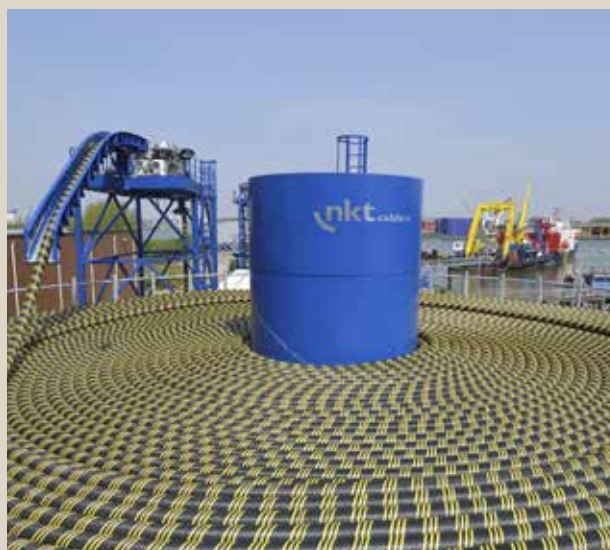
A high-voltage submarine cable waiting to be loaded onto a cable-laying vessel, at NKT Cables' Logistics Centre at Rotterdam, the Netherlands
