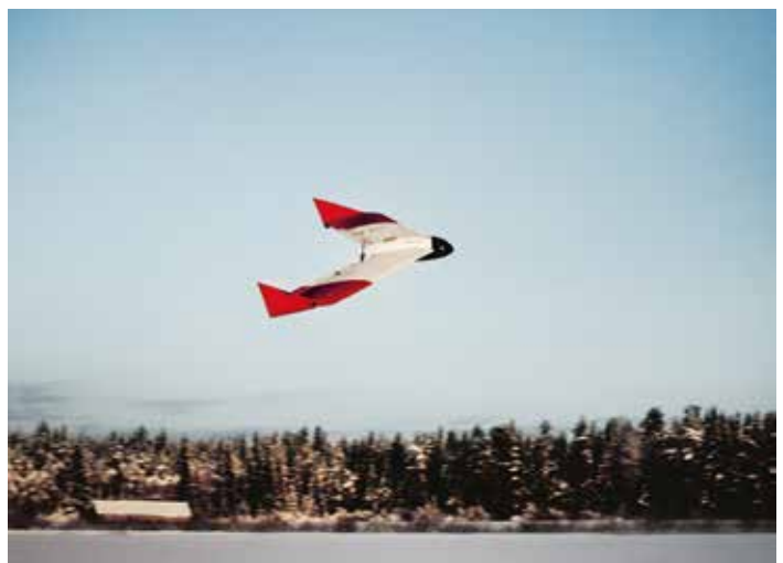
Drones provide quick answers to mining industry. The use of pilotless planes – "drones" – is increasingly prevalent in society. Drones complement traditional measuring methods – compared with helicopters, they are inexpensive and quick to get into the air. Sweco, for example, flew drones over LKAB's mines to calculate the volume of gravel residue. Other areas of application are wildlife monitoring and consequence analyses for forests following storms or fires.
