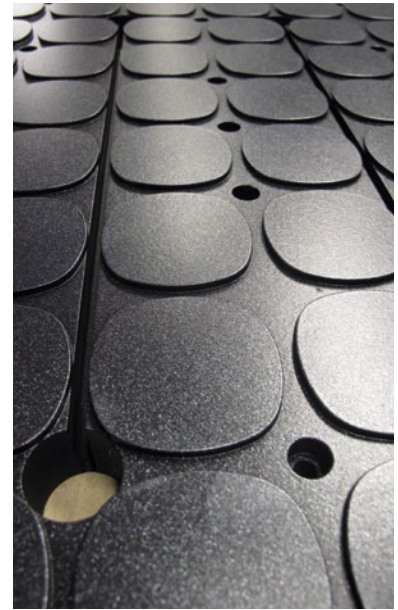
Non stick coated welding tool
