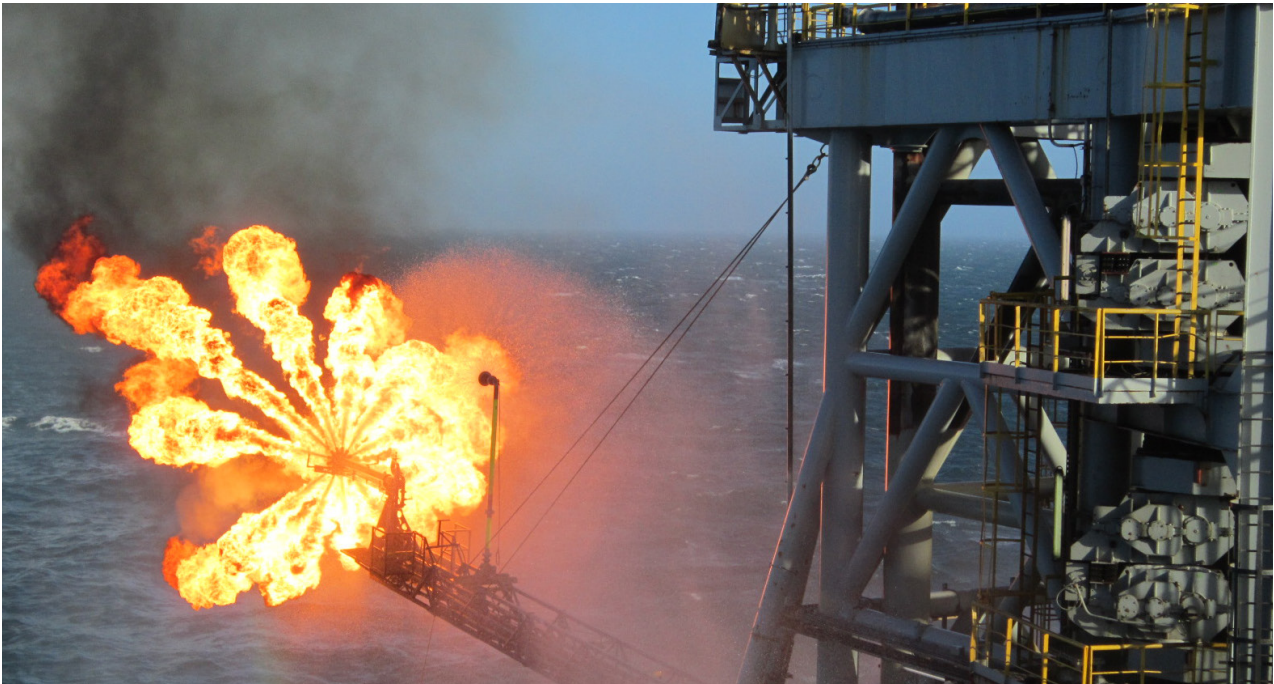
Appraisal well Lille John 2 in Denmark flowed at rates up to c. 1,400 barrels of oil per day, shown here during the drill stem testing operation in which oil produced during the short term test is flared.
