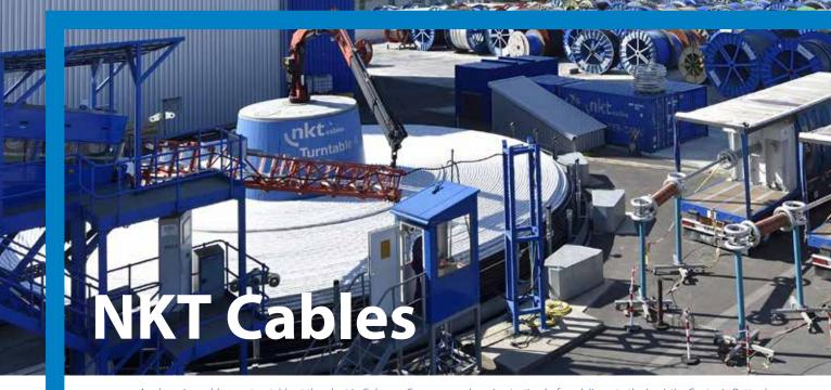
A submarine cable on a turntable at the plant in Cologne, Germany, undergoing testing before delivery to the Logistics Centre in Rotterdam,
