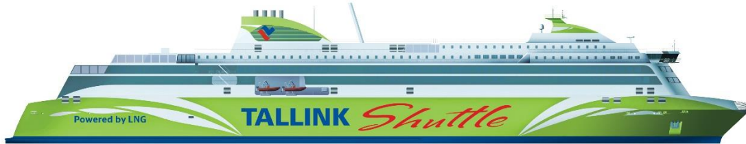
LNG powered fast ferry for the Tallinn-Helsinki shuttle service
