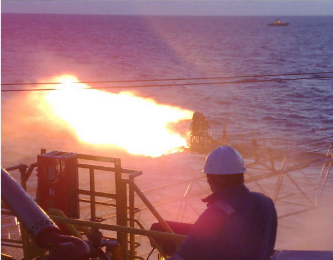
Offshore worker looks on as the 50/11-3 Hook Head appraisal well flows to surface during initial well testing operations
