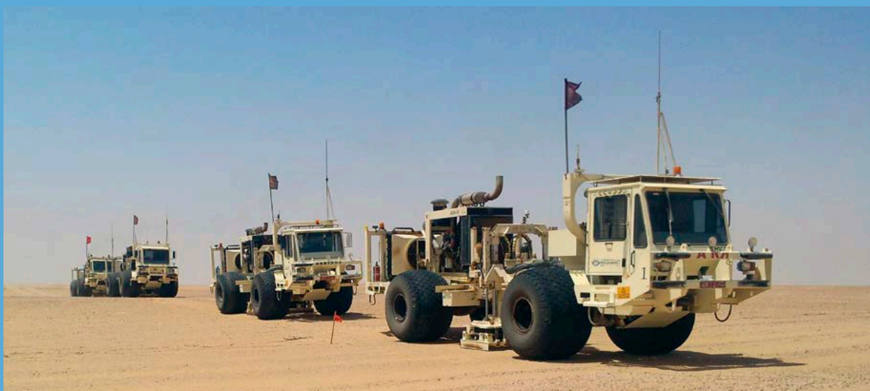
Vibrator trucks at Blocks 3 and 4
