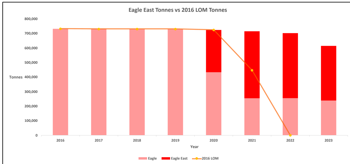
Figure 5 – Combined Eagle East and Eagle mine production plan and contained nickel and copper metal produced in concentrate compared to the current Eagle mine Life of Mine plan.
