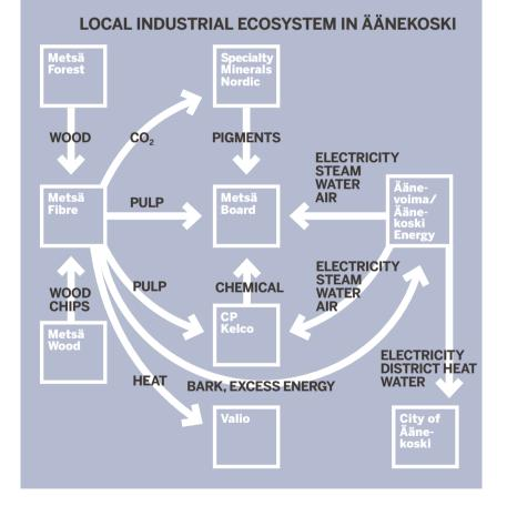
The running mill integrate in Äänekoski, Finland, is a prime example of a vibrant industrial ecosystem. At the same site operates several companies, including Metsä Fibre's mill that supplies pulp to the neighbouring Metsä Board paperboard mill. Metsä Wood is building a peeling line at the site, and the company has a plywood mill less than 10 kilometres away.
