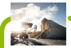
Production side streams are loaded on a truck. The truck heads to the **on-site bioenergy plant** where the side stream is utilised for energy. Another truck drives to a partner company where our side stream is the main raw material.
