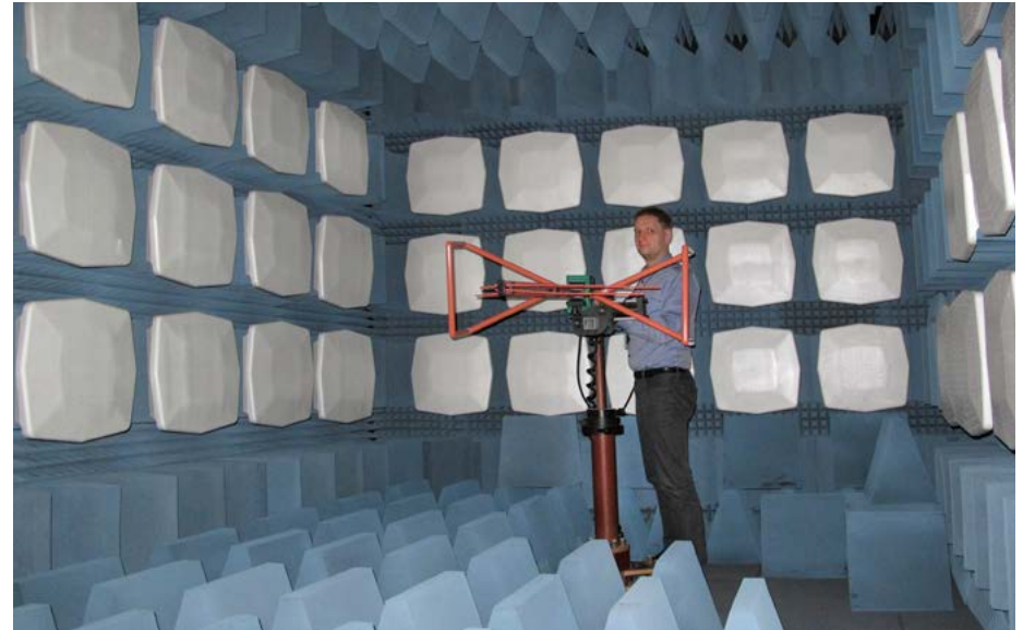
Teleste's Senior Designer / EMC Mikko Nurminen is conducting electromagnetic compatibility (EMC) measurements in laboratory conditions at Turku University of Applied Sciences.
