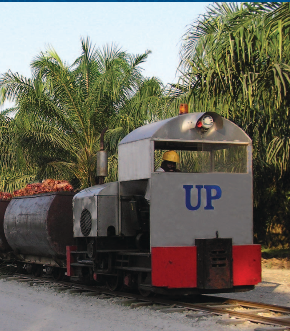
UPB's unique light railway system showing a diesel locomotive pulling a train of fruit cages containing fresh fruit bunches. UPB's railway system stretches over 500 km and is one of the main reasons for its superior quality crude palm oil.
