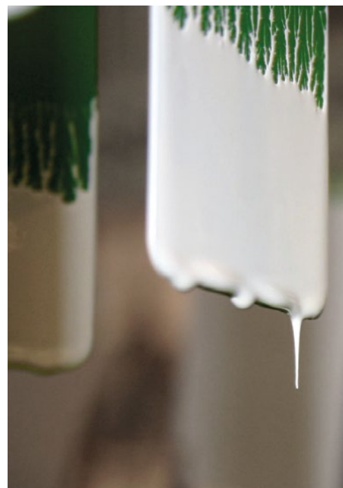
Paint does not adhere to non-stick coatings from Acccoat.
