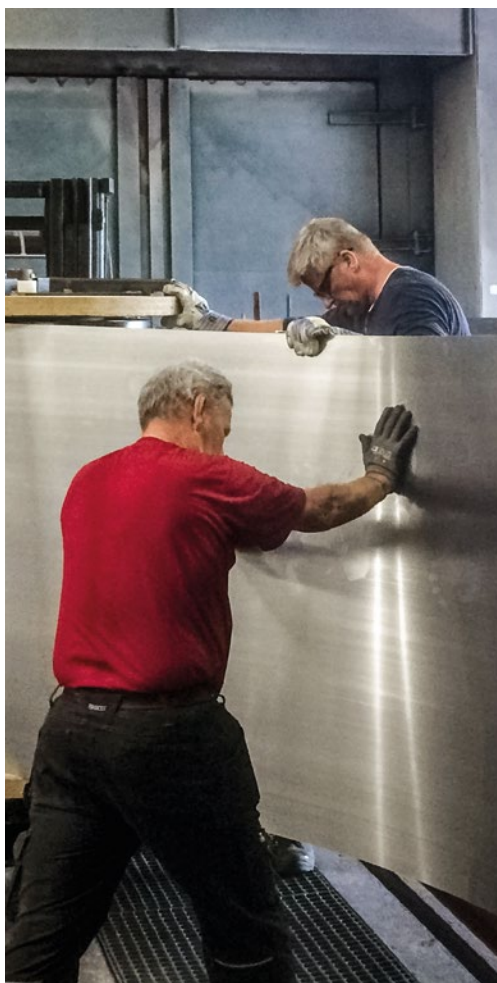
Mogens Hansen and Tommy Petersen preparing surface coating of a 31 metre long steel band to be used in a bakery oven.
