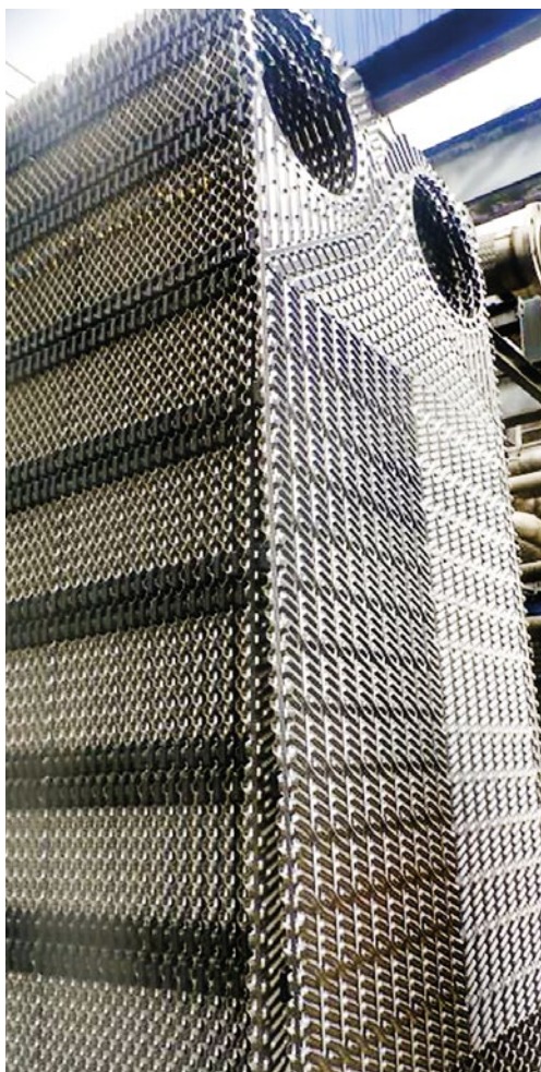
Plate heat exchangers coated with Accolan for improved efficiency and longer lifetime.
