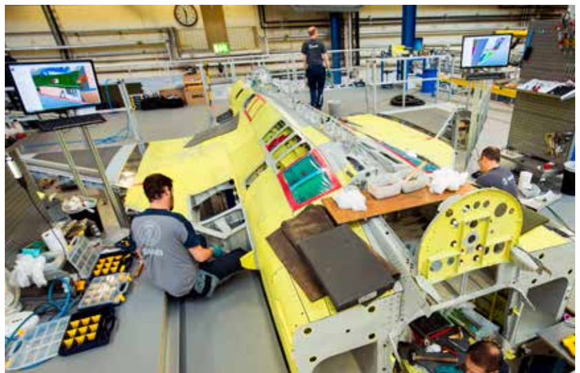
The first test aircraft under construction in the development of Gripen E.
