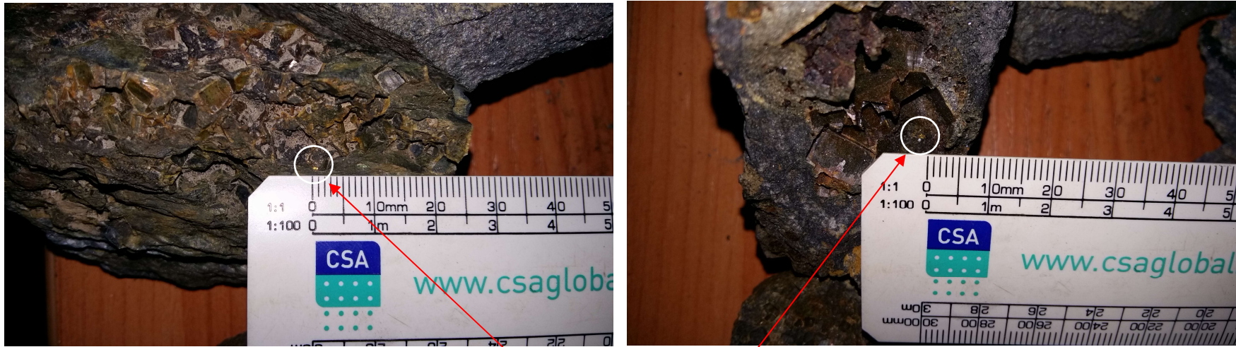
Figure 8. Pictures with visible gold grains in the trench samples (trench #143602)
